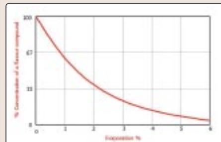
Figure 2: Reduction of a typical volatile by atmospheric boiling assuming liquid-vapour equilibrium which gives the best possible gradient.
