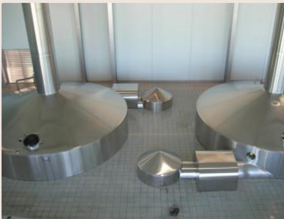
Fosters Brewing Group Yatala Brewhouse showing a top view of the two 800 hl kettles with the tangential entry from the top of the external wort heaters.
