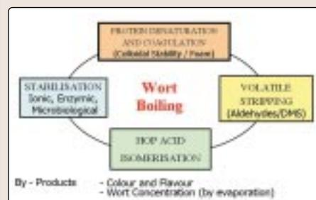
Figure 1: Evaporation tends to be the only process control parameter set by brewers to define effective boil – regardless of boiling technology.
