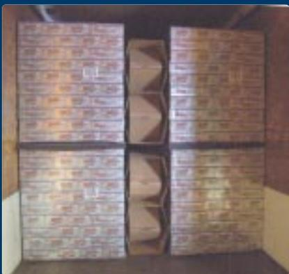
The rather gloomy inside of rail car showing four pallets on slip sheets and a sturdy cardboard support spacer to prevent any movement.
