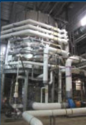
One of the mash vessels. Note the 18" diameter mash main to the lauter on the right.
