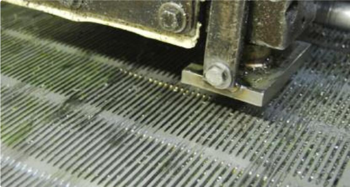
The machine which precisely cuts the slots in the lauter tun plates.
