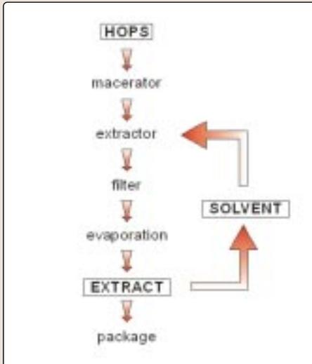
Figure 4. Process flow chart for the manufacture of hop extracts.
